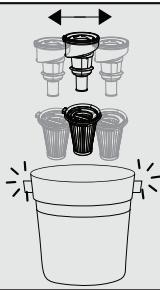
Remove the dust on the pre-filter and the plastic filter by tapping it on a hard surface such as a waste bin or by using a brush.
